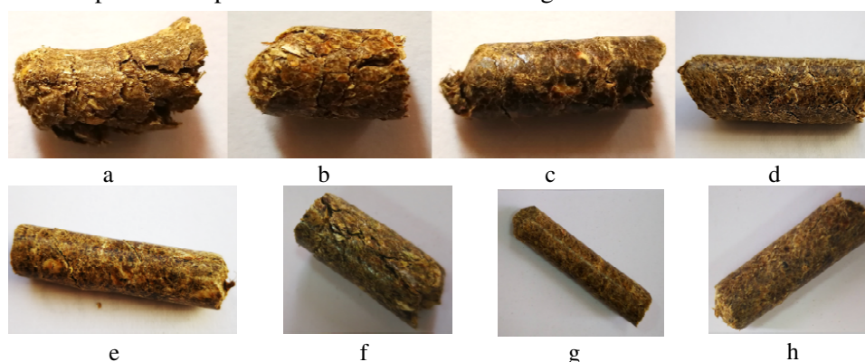
Fig. 2. Overall aspect of pellets obtained: a – wheat straws; b – rapeseed stalks; c – corn stalks; d – wheat straws + rapeseed stalks; e – wheat straws + paraffin; f – wheat straws + paraffin + corn starch; g – wheat straws + rapeseed stalks + corn stalks + dolomite; h – wheat straws + rapeseed stalks + corn cobs
